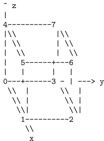
Curved high order  $P_k$  hexaedra ( $k \geq 1$ ) in 3d geometries are supported. These hexaedra have additional edge-nodes, face-nodes and internal volume-nodes.
