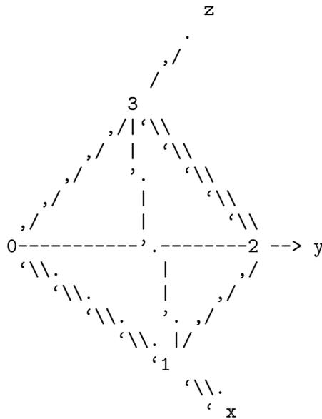
Curved high order  $P_k$  tetrahedra ( $k \geq 1$ ) in 3d geometries are supported. These tetrahedra have additional edge-nodes, face-nodes and internal volume-nodes.
