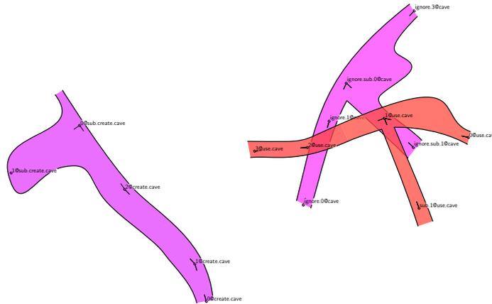
This is because in top level import command, survey *create* is imported from file *create/create.3d* with wrong coordinates, and we import top-level .3d file with *-surveys use* switch. This means, *cave.create.1* will be imported here as *create.1@cave* and not *1@create.cave*.
