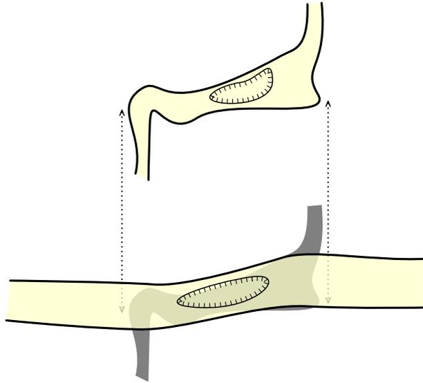
Joining arrows are created from *map-connection* points specified in scraps that are moved. Otherwise these points are ignored.
