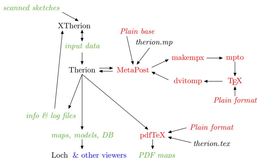
DON'T PANIC! When your system is set-up right the majority of this is hidden from the user and all necessary programs are run automatically by Therion.
