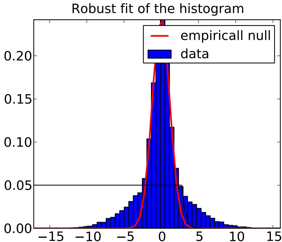
The threshold evaluated with the `ENN.threshold()` method is around 2.8 (using the default p-value of 0.05). The `ENN.uncorrected_threshold()` return, for the same p-value, a threshold of 1.9. It is necessary to use a higher p-value with uncorrected comparisons.
